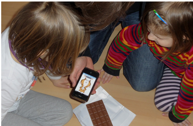
Figure 5: The bar code of the chocolate bar is evaluated by the smartphone, the EAN is sent to our web service and the corresponding hamster visualization (see also Figure 4) is immediately shown on the display. The wrapping was removed to anonymize the product.
